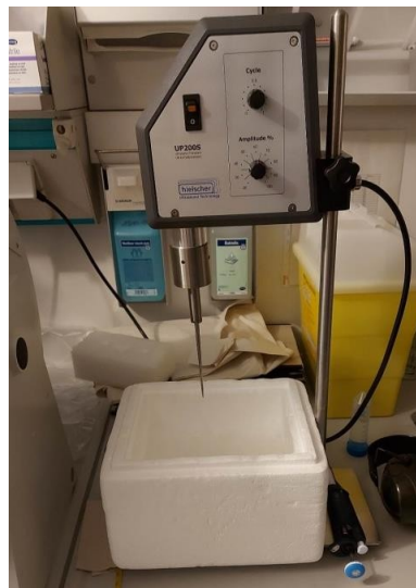
Figure 10. Working system used in sonication-assisted decellularization methods
