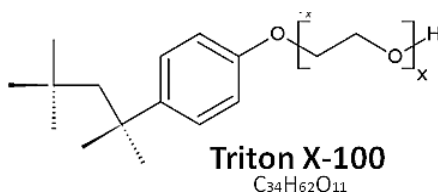
Figure 5. Structure and formula of Triton X-100 [143]
