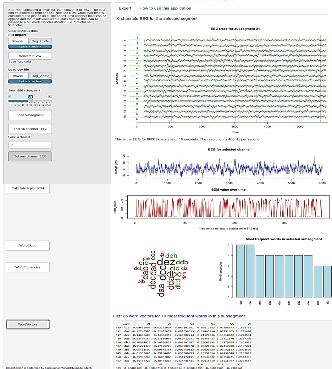
Figure 7.22. Graphical User Interface (GUI) to analyze the algorithmic complexity of EEG using ISAAC-EEG-BDM-NLP/Word2vec_2.1.0 software.
